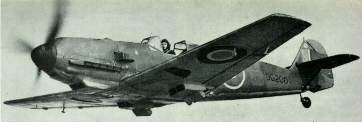
A captured E-4 under test by the R.A.F. Radiator flaps and balance horns are clearly visible. (Photo: Imperial War Museum)
