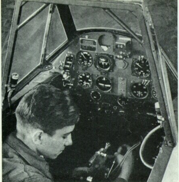
A fitter wires up the firing button of a Bf 109E-4. The gun-sight head with reflector has not yet been installed, although the selector box can be seen at the top of the instrument panel.
