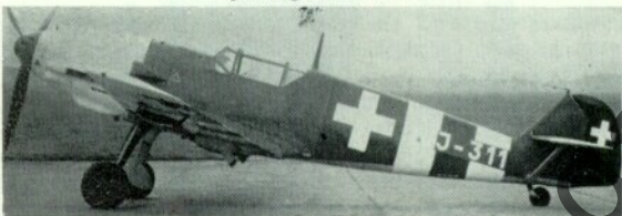
Above: J-311, Bf 109E-3 W.Nr.2159, in the colourful fuselage markings of the Swiss Air Force. This machine was written off on 28th December 1949.
